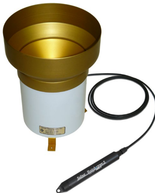
Figure 10-21 Rainlogger 5 Connected to Tipping-bucket
